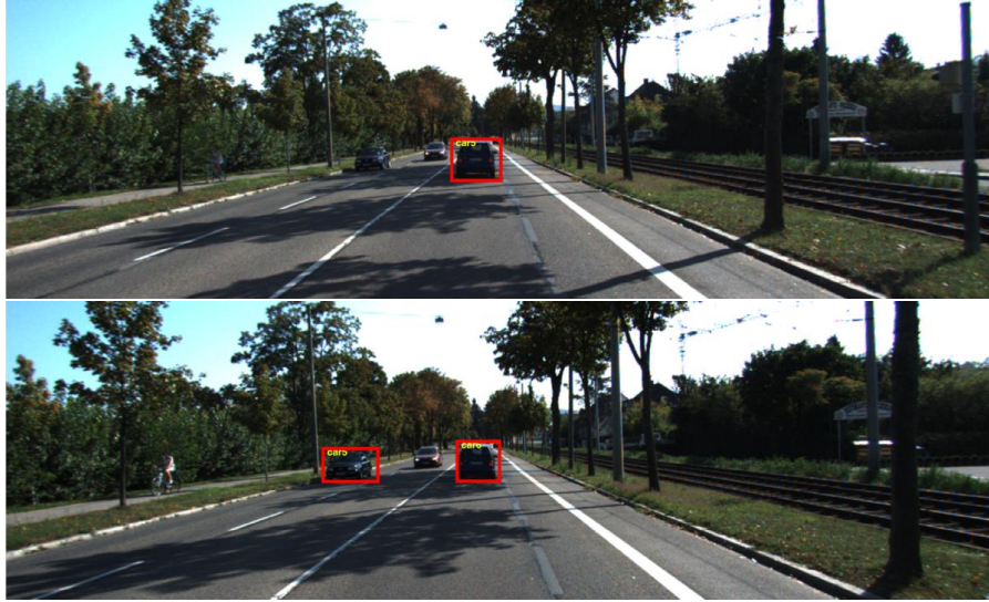
Figure 3: When there are two cars with similar color, the Histogram of Color method has a bad performance.
